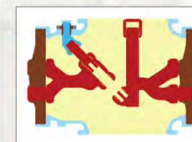
Disconnector opened with earthing switch closed
