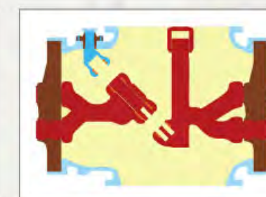
Disconnector opened with earthing switch opened
