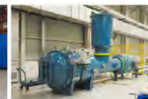
Insulator testing fixture
