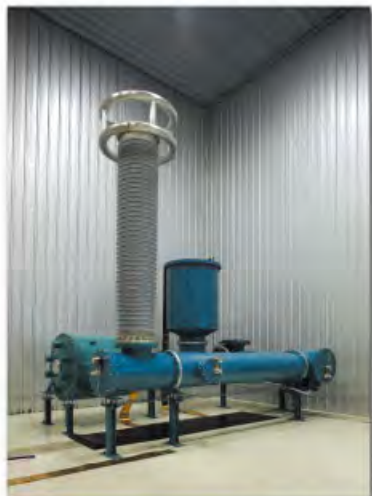
Test transformer, coupling capacitor and impulse voltage lead-in bushing and 1,500kV impulse voltage generator
