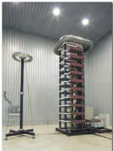
Test transformer, coupling capacitor and impulse voltage lead-in bushing and 1,500kV impulse voltage generator
